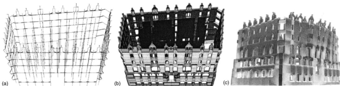
Figure 2.5: Multiple system: (a) Wire representation of the inner and exterior walls; (b) representation of floor slabs as a grillage; (c) predicted deformed shape amplified for the earthquake acting transverse to the main façade, [Roca *et al.* (2005)].
