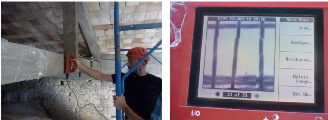
Figure 5.29: Pacometer testing of truss beams in San Domenico Church (courtesy of EXPIN).
