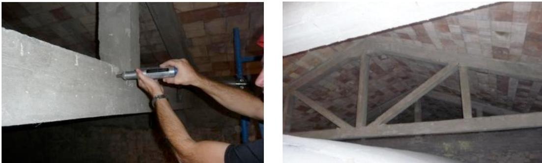
Figure 5.26: Classification of concrete strength by Schmidt hammer on San Domenico roof trusses (courtesy of EXPIN).
