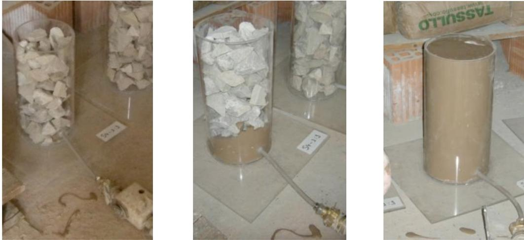
Figure 3.9: Injectibility test and preparation of the cylinders.
