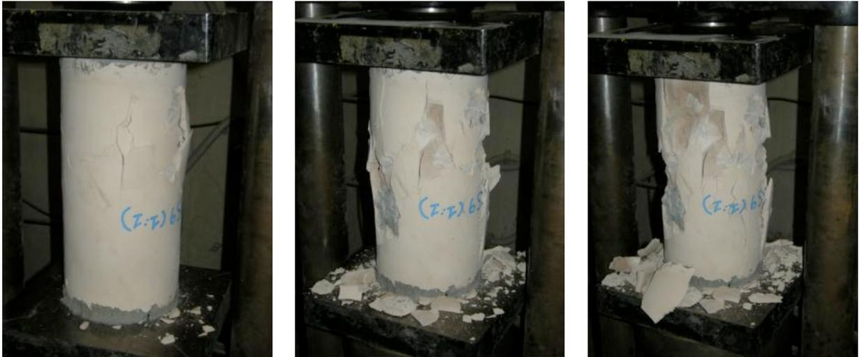
Figure 3.14: Progress of the compression test for a grouted cylinder.
