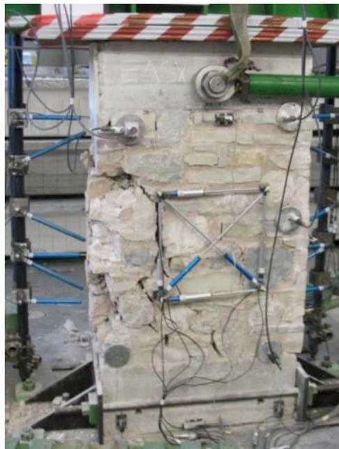
Figure 4.35: Stone masonry wall during shear-compression test experiencing the formation of big cracks.
